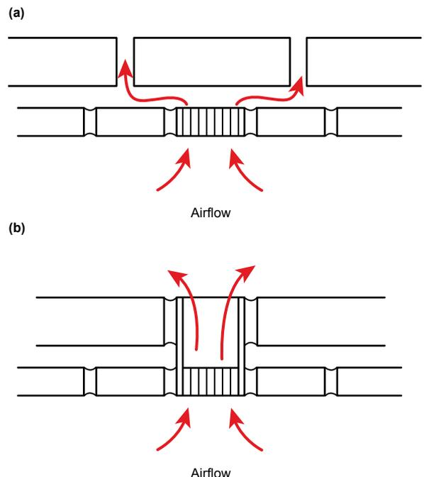
Figure 4: Airflow through (a) an unsleeved vent through cavity wall, (b) a sleeved vent through cavity wall
