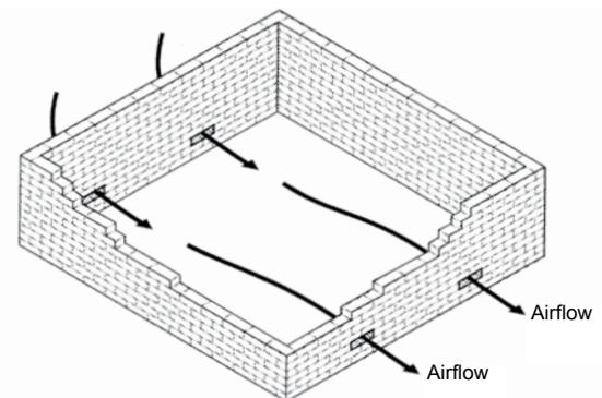
Poorly located airbricks cause areas of poor ventilation (dead areas)
