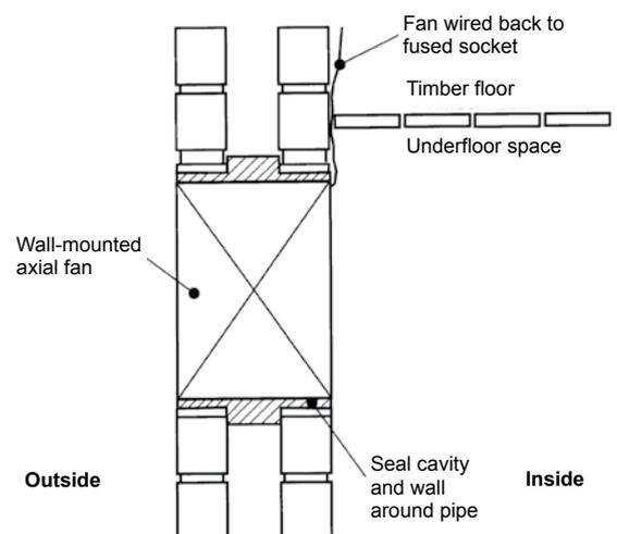
Figure 10: Axial flow fan located within the thickness of a cavity wall
