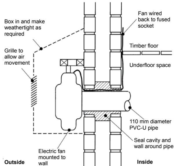
Figure 8: In-line duct fan with pipe fixed to a cavity wall
