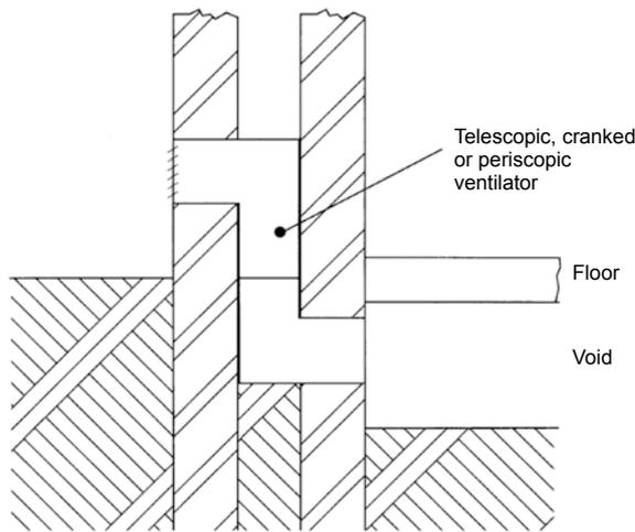
Figure 6: Section through a telescopic vent
