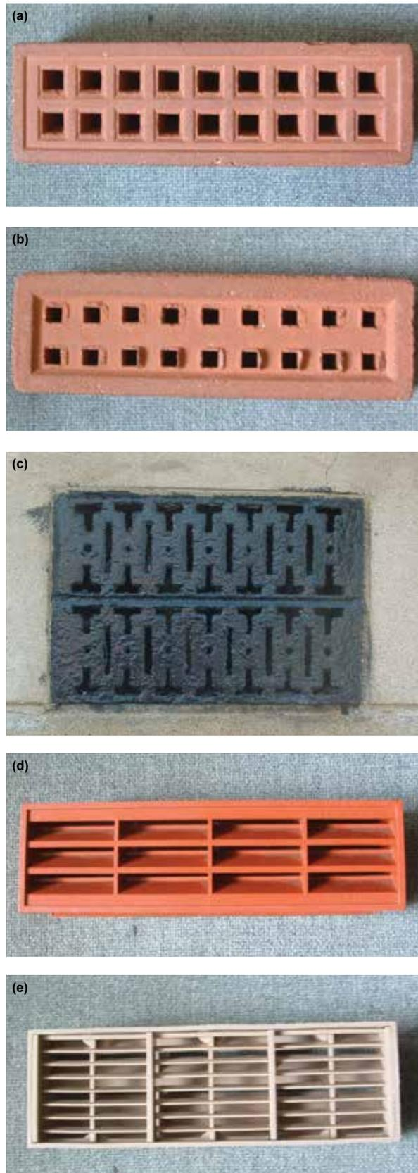
Figure 5: (a) front and (b) rear of a terracotta air brick showing actual open area is less than half what it appears from the front, (c) typical cast iron vent, (d) and (e) modern plastic ventilators offering more open area than a similar-sized terracotta air brick
