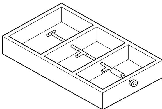
Figure 12: A manifolded system beneath three rooms fitted with a silencer close to the fan
