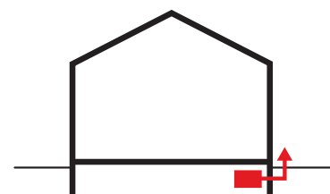
Externally constructed sump with low-level exhaust
